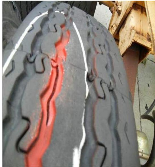
NOTE: Neither the length of the split, nor the number of splits is of consideration. *The **sole consideration on whether the tire is to be removed from service is the depth of the splits.*** Splits in the channels of the tire should be carefully probed to determine if there is exposed cord. If the cord is exposed, either visually or it can be felt with a probe, the tire should be removed for service. If the cord cannot be felt or seen visually - the tire is to be left on the chassis.
