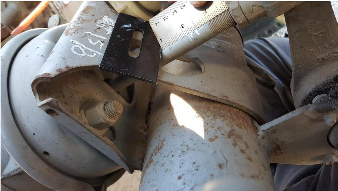
NOTE: It is also acceptable to measure from the straight edge in the brake-applied position to the brake released line.
